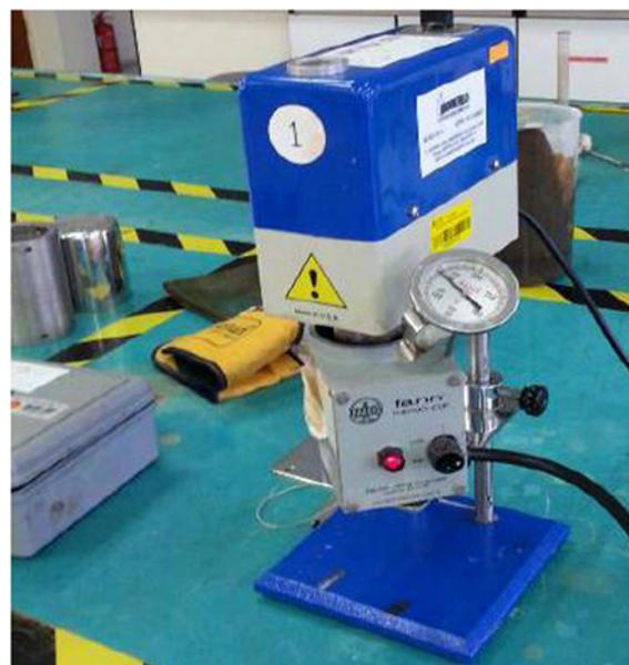
**Figure 1** Fann rheometer with Baroid hot cup.
