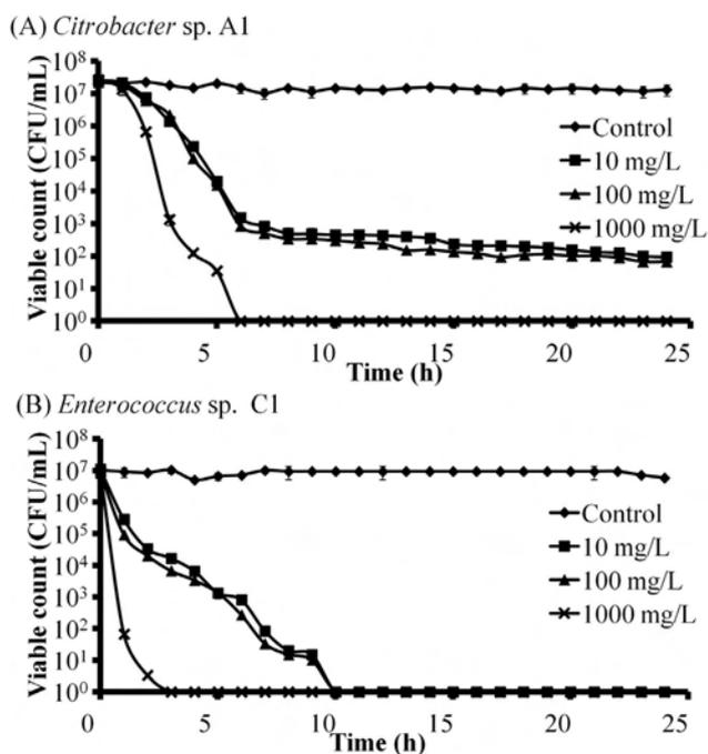
**Figure 7.** Antibacterial effect of AgNPs at concentrations 10–1000 mg/L on (A) *Citrobacter sp. A1* and (B) *Enterococcus sp. C1* in 0.1M PB (pH 7) at 30°C with shaking at 200 rpm. AgNP = silver nanoparticle; CFU = colony-forming unit; PB = phosphate buffer.
