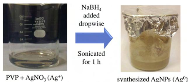
**Figure 1.** Change in the color of PVP-AgNO<sub>3</sub> solution from clear to yellow, indicating a reduction of Ag<sup>+</sup> to Ag<sup>0</sup> during synthesis of AgNPs. AgNP = silver nanoparticle; PVP = polyvinylpyrrolidone.
