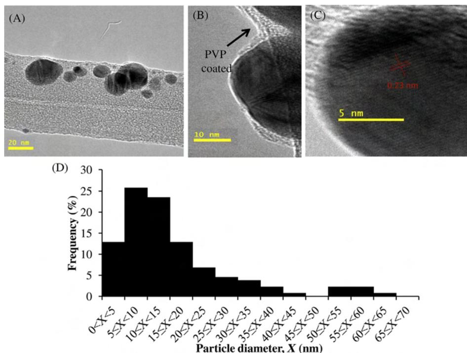
**Figure 5.** TEM images of AgNPs: (A) at 100,000 $\times$  magnification, (B) at 250,000 $\times$  magnification, and (C) at 500,000 $\times$  magnification, and (D) histogram of particle size distribution. AgNP = silver nanoparticle; PVP = polyvinylpyrrolidone; TEM = transmission electron microscopy.
