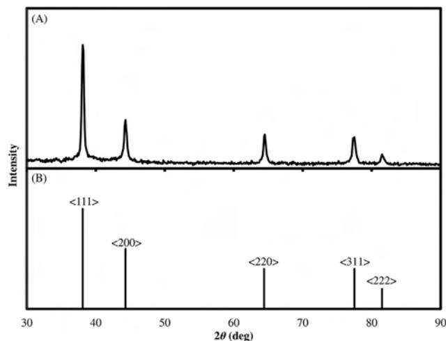
**Figure 4.** XRD pattern of (A) AgNPs and (B) pure silver with FCC symmetry (JCPDS file no. 04-0783). AgNP = silver nanoparticle; FCC = face-centered cubic; JCPDS = Joint Committee on Powder Diffraction Standards; XRD = X-ray diffraction.
