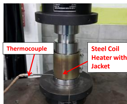
Figure 2 Briquetting process using Instron Machine 600dx
