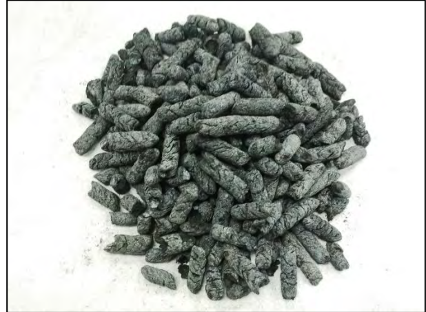
Figure 2b Biochar of OPEFB briquettes after gasification
