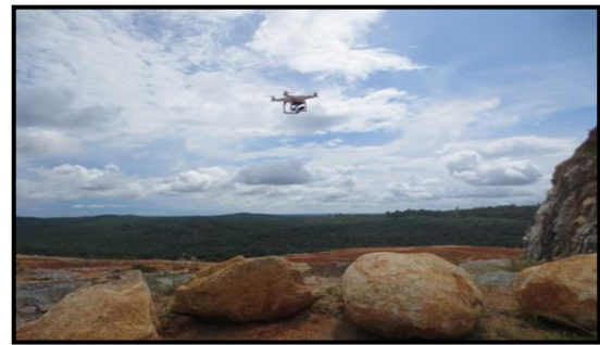
Figure 3 Unmanned Aerial Vehicle taking aerial photographs in granite quarry [52]
