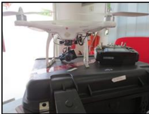
Figure 2 Unmanned Aerial Vehicle (UAV) with Canon camera and remote control [52]
