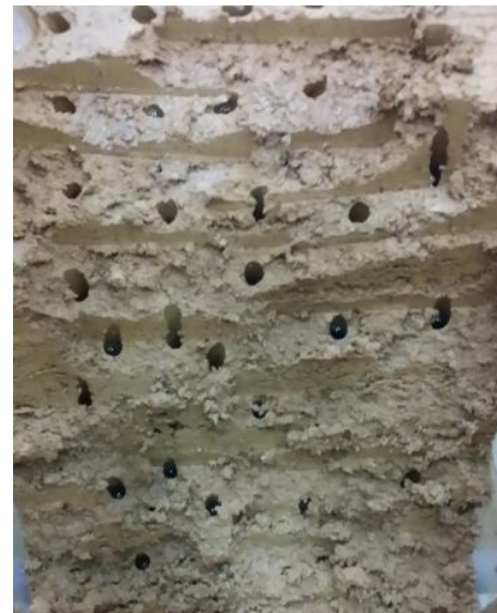
Figure 4 Infiltrating water hold in the burrow hole
