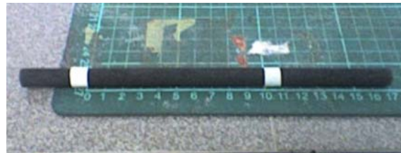
Figure 4 A 210 mm propellant rod with markers 100 mm apart
