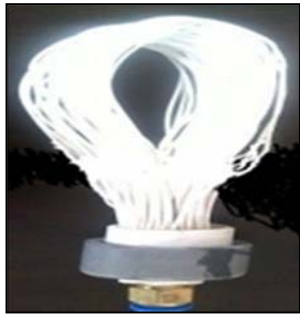
Figure-1. U-shape ultrafiltration membrane module.
