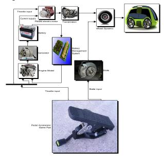
Figure 2 Series hybrid electric vehicle simulation model
