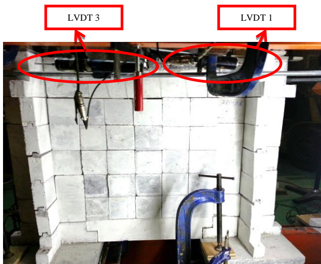
Figure 2(a) Instruments Set Up for Push Over Cyclic Test (Rear View)
