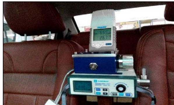
Figure-4. Setup of TVOC instrument and Tolaire 7001.
