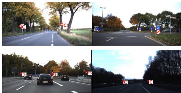
Figure 11 TS detection and shape matching samples (C is for Circle TS and S is for Stop TS)
