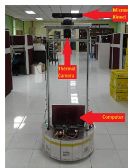
Figure 1 UTMbot-Mobile Robot used in this work
