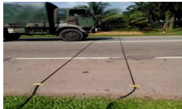
Figure 2 Pneumatic Tubes are 1 Metre Apart
