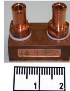
Figure 1 Tested microcooler with structured area
