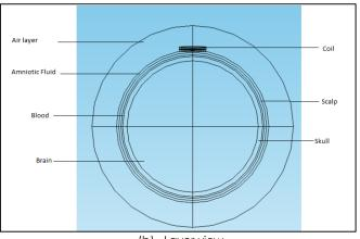
(b) Layer view Figure 3 MIS setup in COMSOL Model
