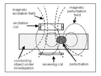
Figure 2 Basic MIS setup [13]
