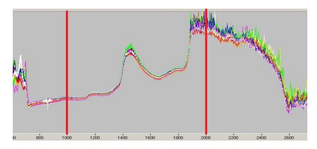
Figure 4 The absorption wavelength chose as the input source from 1000nm until 2000nm
