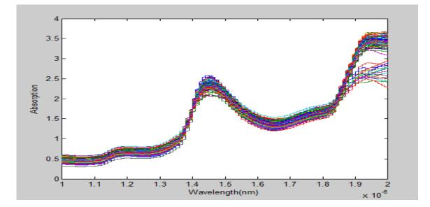
Figure 7 The processed signal data at fingertip using the Savitzky-Golay Filter
