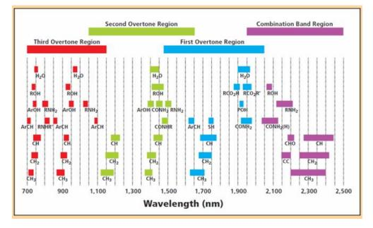
Figure 5 The spectral region of the near-infrared wavelengths
