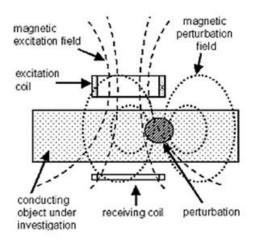
Figure 2 The principle of MIT [19]
