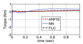
Figure 9 Control signal for step input
