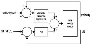
Figure 6 TWIP control scheme
