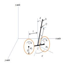
Figure 5 Schematic diagram of TWIP
