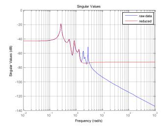
Figure 7 Sigma plot reduced order system
