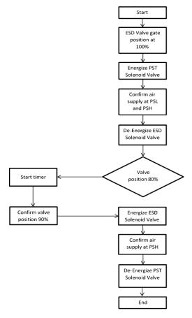
Figure 2 Process flow for partial stroke testing
