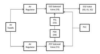
Figure 1 Block diagram for partial stroke testing
