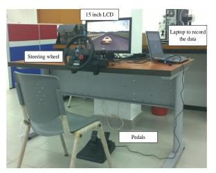
Figure 4 The hardware setup for this experiment
