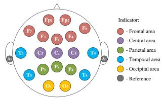
Figure 1 10-20 Electrode placement system with  $A_1$  and  $A_2$  references
