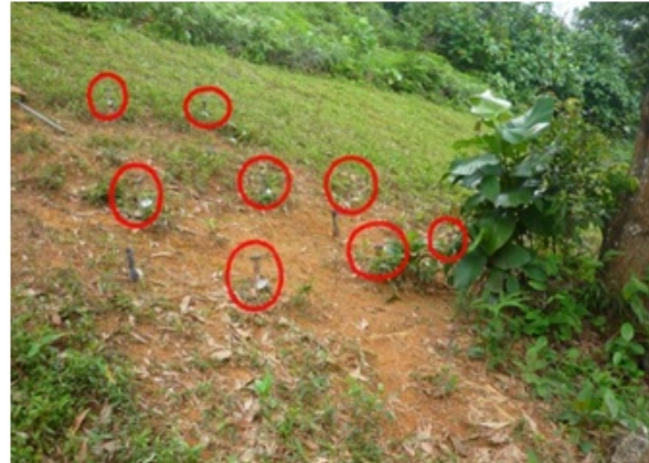
Figure-2. Tensiometer installed at slope.
