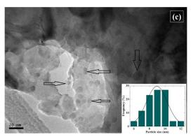
**Figure 3 (a)** FESEM image at specific region of glass sample containing 0.4 mol% Au; **(b)** the respective EDX spectra of glass sample; **(c)** TEM image of the Au NPs (glass containing 0.4 ml% Au) show closely dispersed particles, majority with non-spherical shape. Inset shows histogram of Au NPs with average diameter of  $\approx 9$  nm
