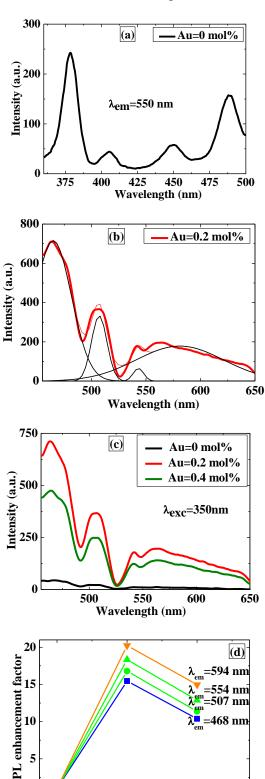
Figure 4 (a) Excitation spectrum of the glass samples in range of 360 to 500 nm; **(b)** PL spectra for glass containing 0.2 mol% Au with Gaussian fit; (c) Luminescence spectra for all samples under 350 nm excitations; (d) PL enhancement factor showing enhancement and quencing ratio for respective glass samples with varying Au concentration
