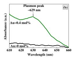
**Figure 2 (a)** UV-Vis-NIR absorption spectra of glass samples in the range of 400–1600 nm; **(b)** SPR band positions of gold NPs
