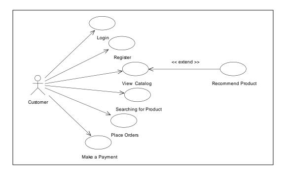
Figure 2. The use case diagram for customer's view
