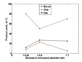
Figure 5: Effect of microwave absorber on yield of OPF microwave pyrolysis product
