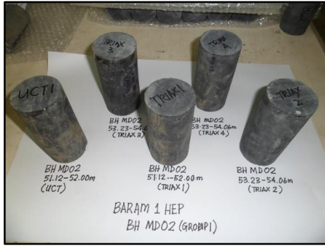
Figure 5 The core samples of shale prepared for laboratory test
