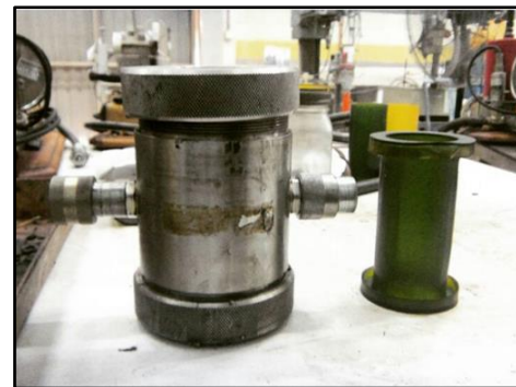
Figure 8 Hoek's cell and sample sleeve for triaxial test
