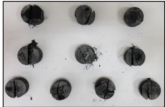
Figure 13 Samples of Shale after Brazillian test
