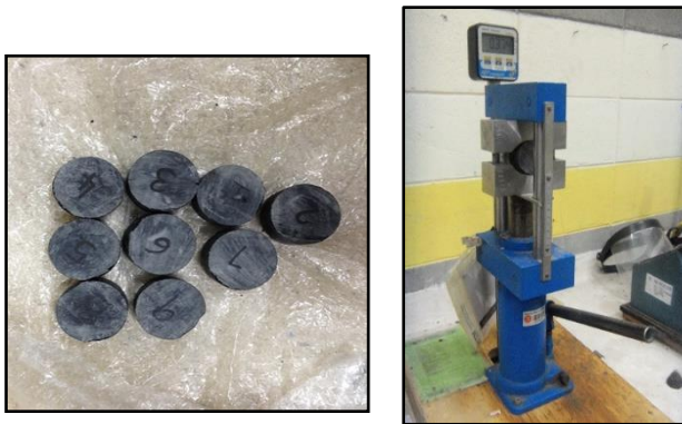
Figure 10 Brazillian test and disc shaped samples
