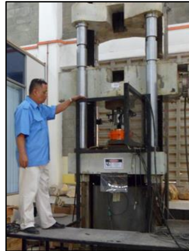
Figure 7 A Universal servo-controlled testing machine
