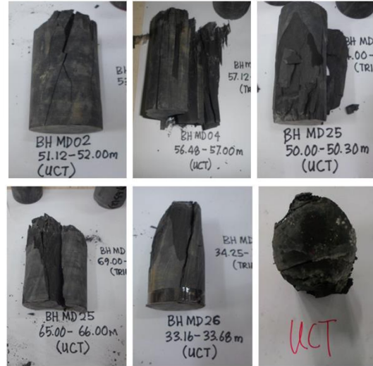
Figure 11 Shale sample after UC T
