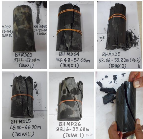
Figure 12 Samples after Triaxial Test
