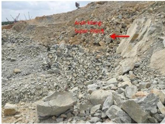
Figure 8 Inspection carried out on site. Red arrow indicates the direction of joint dominance (to the west)
