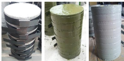
Figure 1 Externally coated specimens; (a) uncoated specimen; (b) ZC coating; (c) MP coating
