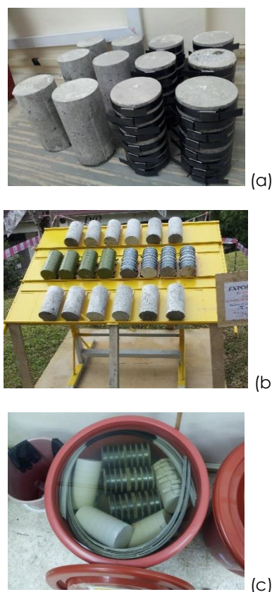
Figure 2 Concrete specimens for (a) indoor exposure, (b) Outdoor exposure, (c) saline water exposure
