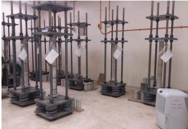
Figure 2: Compressive creep rig with specimen under sustained load
