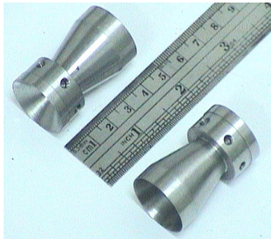
Figure 6 Convergent-divergent nozzle for rocket motor
