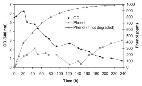
Figure 5 Continuous biodegradation with 1000 ppm of influent concentration
