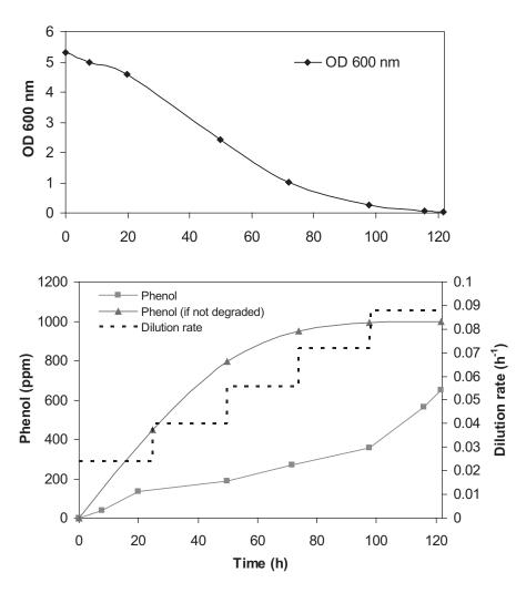
Figure 3 Continuous biodegradation of non-acclimatized microorganisms
