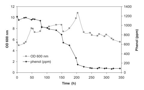
Figure 1 Phenol degradation during acclimatization stage
