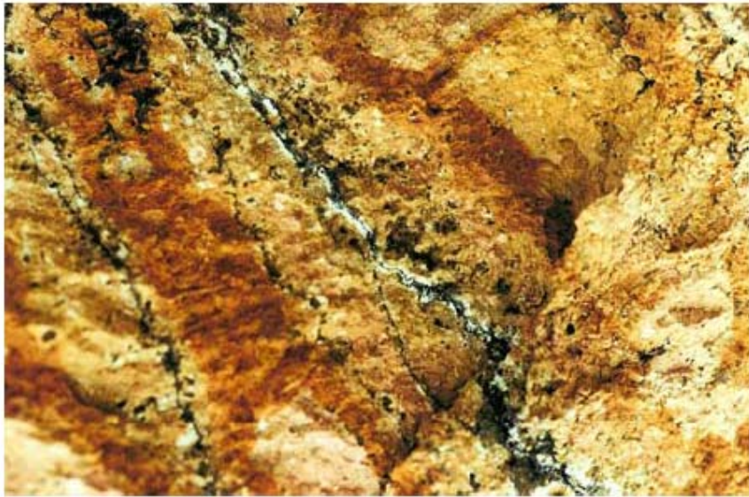
Figure 2.4 Black seams sandwiched within a white clay vein formed along a deformed relict joint plane showing irregular waviness.
