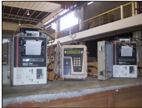
Figure 1.3: The automatic flowmeter (area-velocity ISCO)
