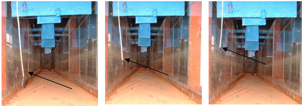
Photo 3.6: Locations of digital thermometer at different depths in the flume
