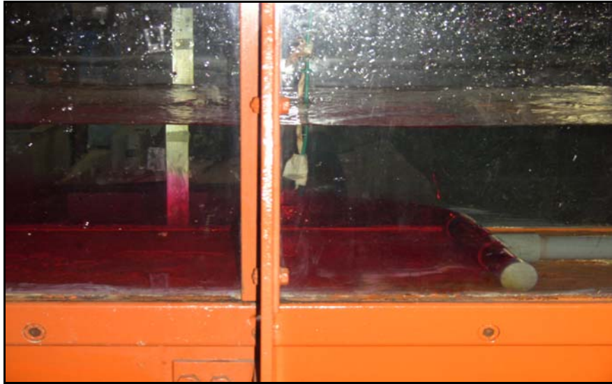
Photo 4.1: Trajectory of thermal effluent discharge in the channel ( Q_e=0.05 liter/s, Q_a=10 liter/s)
