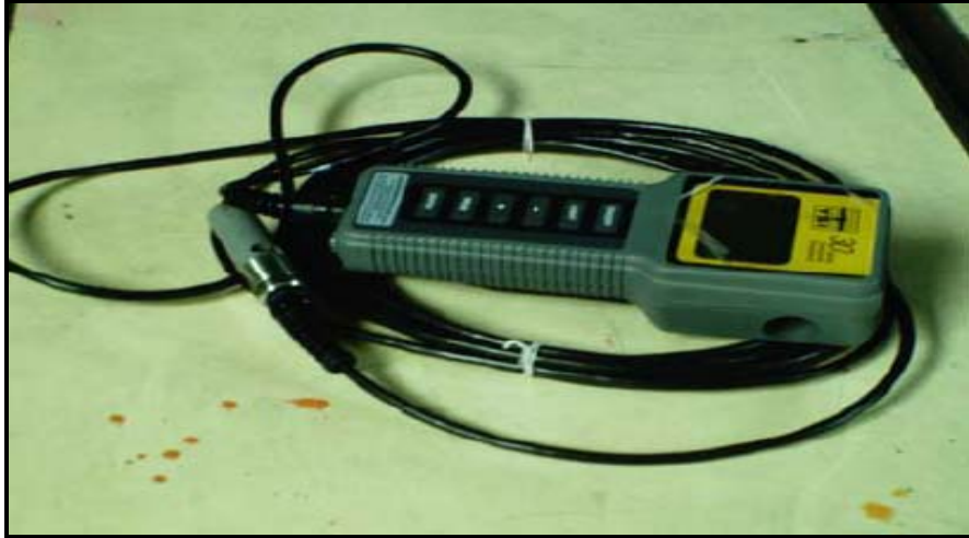
Photo 3.2: YSI 30 Salinity, Conductivity, and Temperature (SCT)
