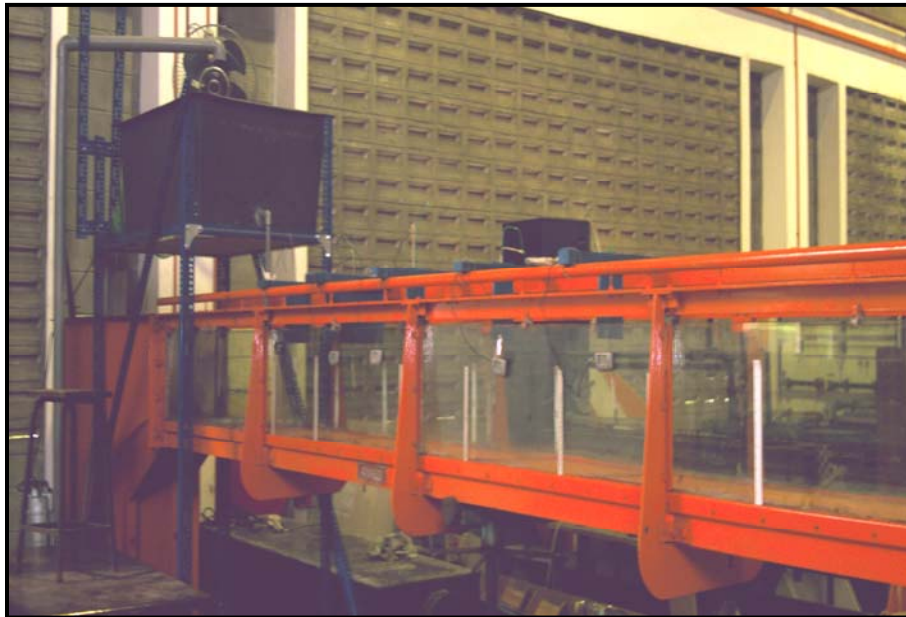
Photo 3.1: 7.0 m long, 0.3 m wide and 0.3 m deep glass flume
