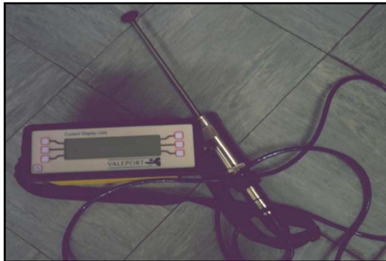
Photo 3.5: 2 axis electromagnetic Valeport current meter model 802
