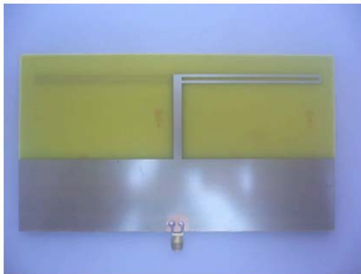
Figure 3.14: Back side photograph of the double sided planar folded dipole
