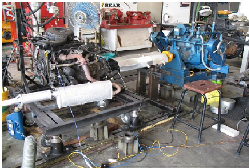
Figure 6: Experimental rig of 660 cc Daihatsu engine with Hydro water break dyno as load factor
