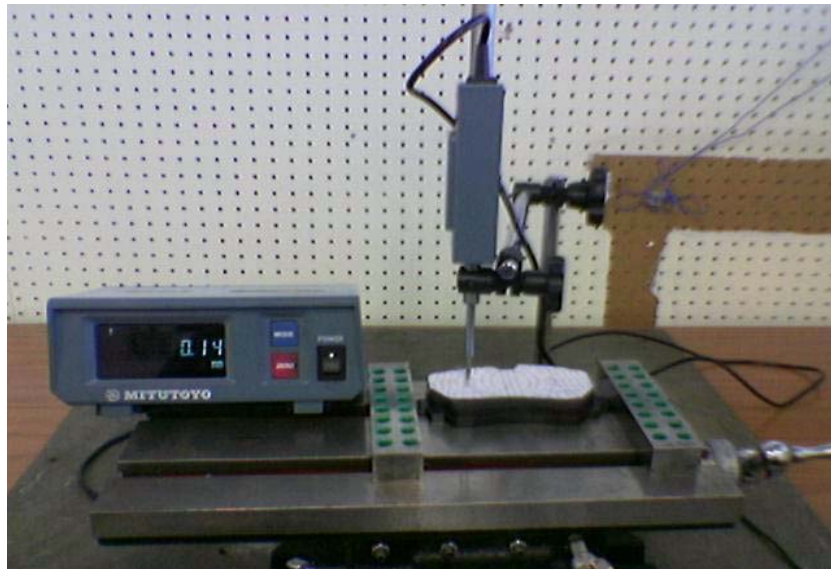
Figure 2: Arrangement of tools for surface measurement
