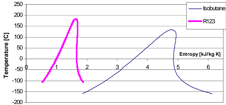
Figure 2: T-s diagram of R123 and Isobutane
