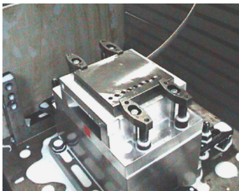
Fig. 1. Workpiece setup on the top of dynamometer.
