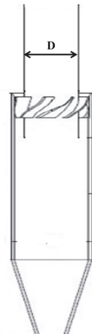
Figure 3. Miniature Cyclone with Axial Entry
