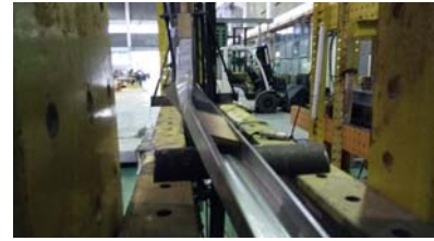
(c) Side view of the failure behaviour on roof truss from left hand side
