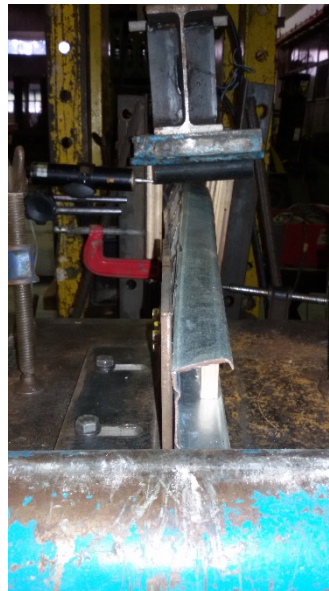
Figure 4: Distortional buckling of curved beam
