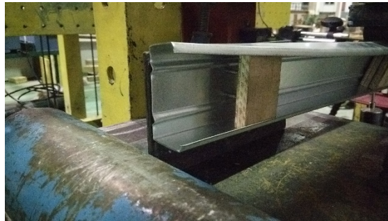
Figure 3: Distortional buckling of straight beam
