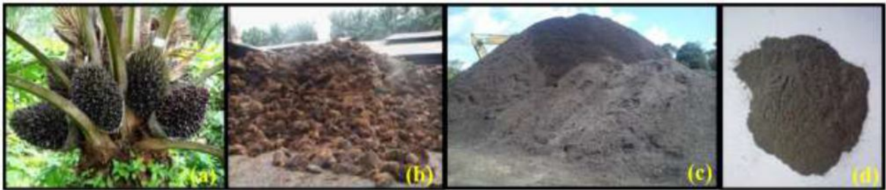
Figure 1: Palm tree (a), fruits bunch (b), POFA (c), and ground POFA (d).
