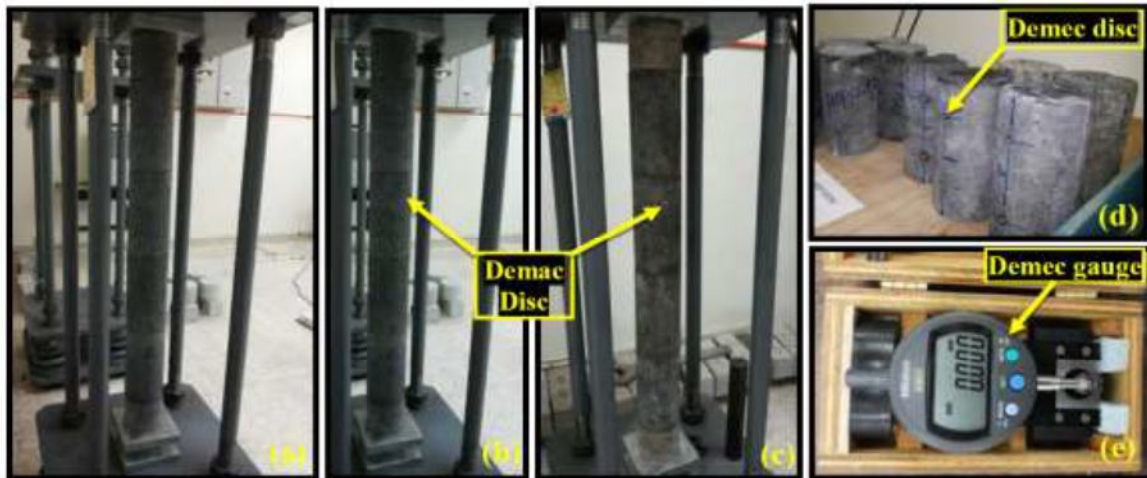
Figure 2 OPC (a), POFA-50 (b), and POFA-70 (c) samples under loading frame for creep measurements, shrinkage specimens (d), and Demec gauge (e).
