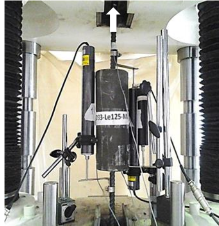
Figure 2: Test setup of tensile load.
