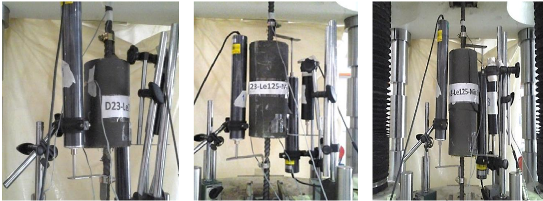
Figure 3: Failure modes; (a) bar bond-slip; (b) bar fracture; (c) grout cover fractured.
