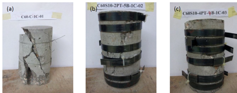
Figure 4: Failure mode of specimen for (a) control, (b) 2-layer confinement and (c) 4-layer confinement
