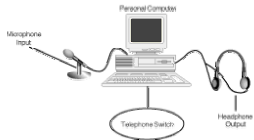
Figure 2.4: Typical unified line TAPI configuration
