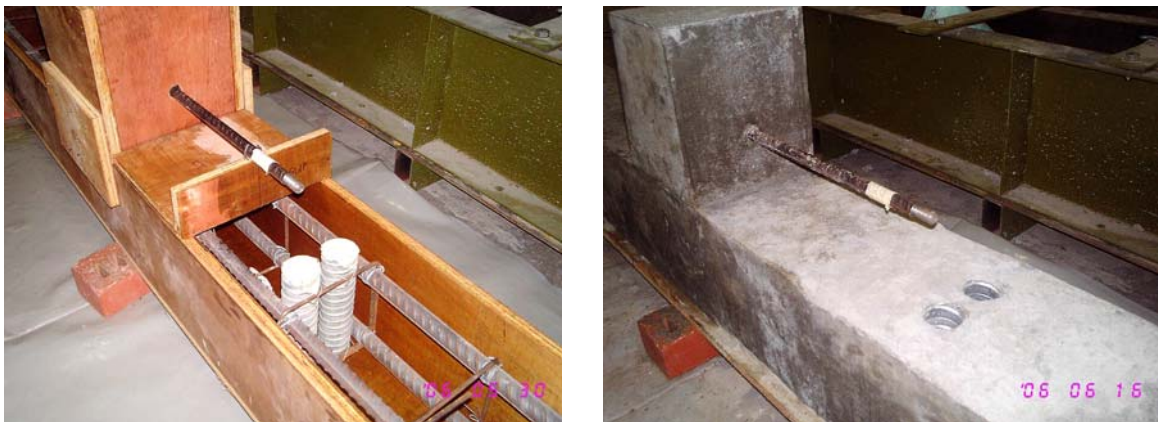
Figure 9 Precast column complete with corbel, projecting dowel bar and two sleeves for precast beam-to-column connection (specimen 4)
