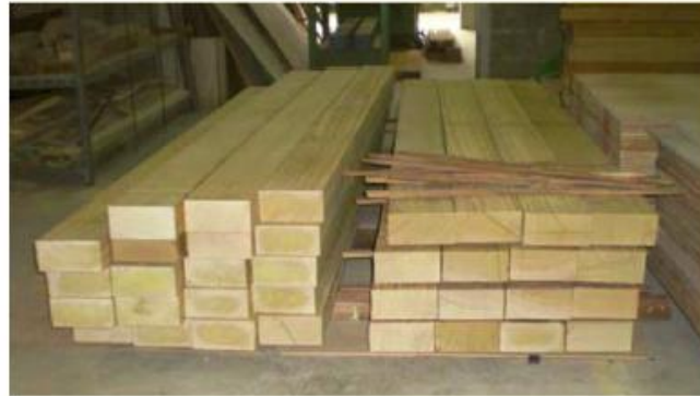
Figure 1: Yellow Meranti timber beams sourced from Malaysian jungles (Yusof, 2010).
